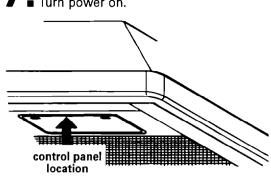
The range hood controls are located in a grey panel on underside of the canopy. To open the panel, press on the front edge of panel and release. The control panel will drop down.
